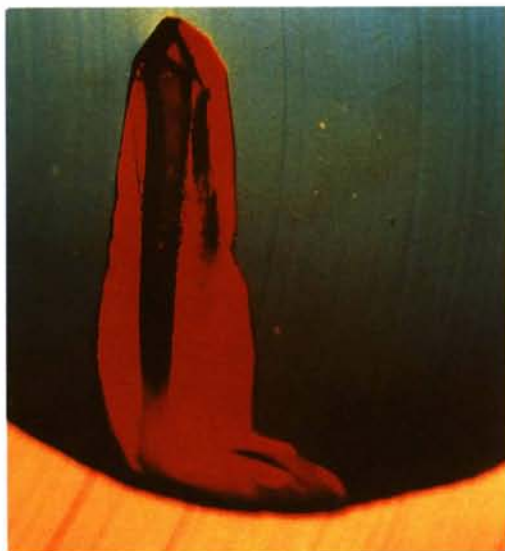
Fig. 1. Crystal of cytochrome c_6 from M. braunii (largest dimension ca 1 mm)
